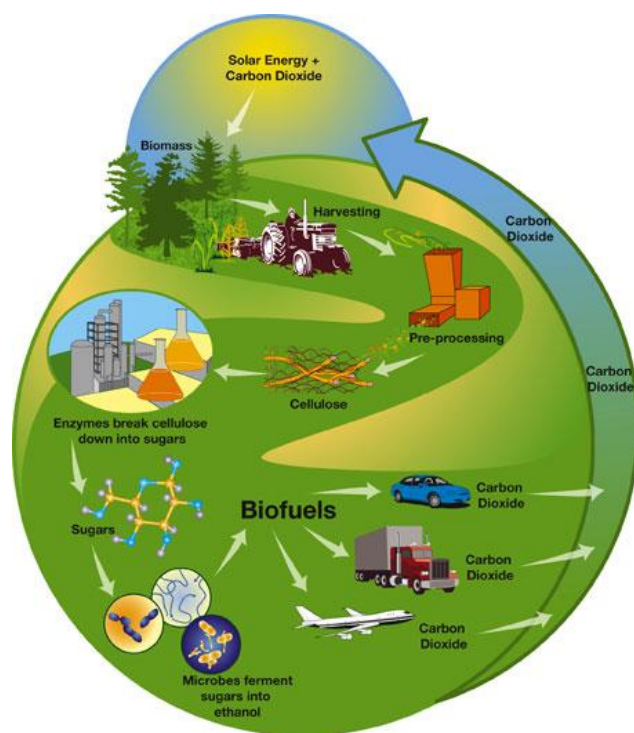
Figure 1.1: Biomass Energy Cycle
